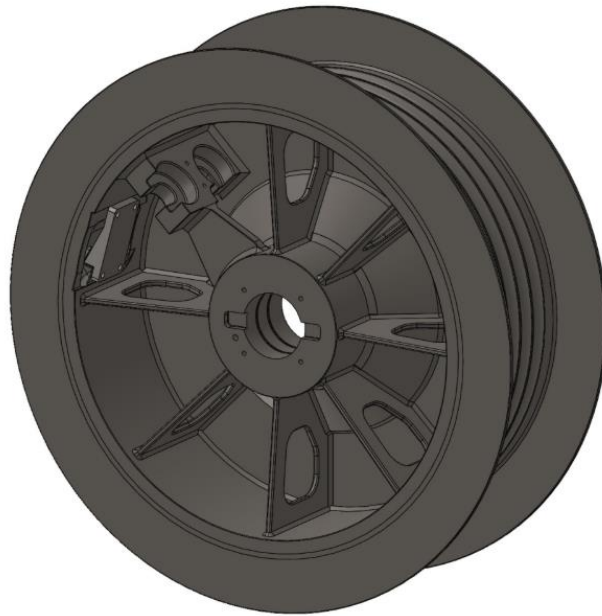
Figure 11. Sheave model – showing stopper insert termination point on the inside of the drum
